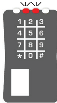
Middle red lights blinking RS485 or managed mode – reader is in sync with Master Unit
